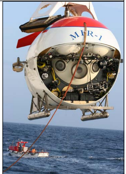
MIR submersible. Capable of depths of 6000meters, the Mir's carry 3 personnel on dives of up to 24 hours.
